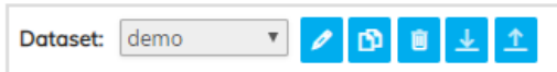
Figure 3.5: The dataset tells you which databook is being edited, and databooks can be renamed, copied, deleted, downloaded or uploaded.
